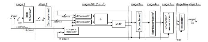
Fig. 1. Top-level design of accumulator architecture. Alpha represents the pipeline latency of de-normalize/addition datapath.
