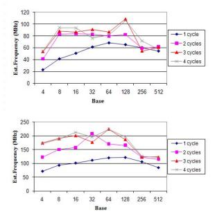
Fig. 2. Synthesis results for Virtex 2 Pro 100 (top) and Virtex-5 LX 330T (bottom), as operating frequency versus base value.
