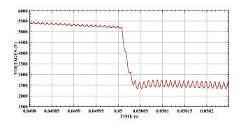
Fig. 14. Single-bus power system analog output, phase 1 zoom.
