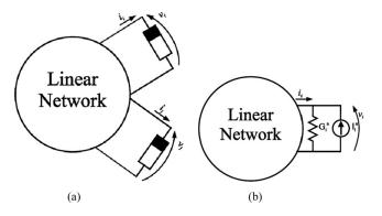
Fig. 1. Linear networks with nonlinear components. (a) With two nonlinear components. (b) With one current-type nonlinear component.
