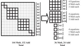
Fig. 4. Separation of subsystems.
