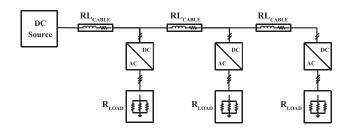
Fig. 9. Single bus shipboard power system.
