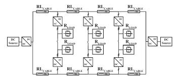
Fig. 10. Dual bus shipboard power system.
