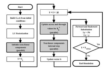
Fig. 2. LB-LMC solution flow.
