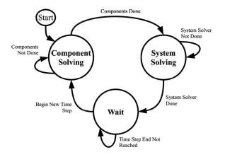
Fig. 7. Finite state machine for multi-cycle simulation engine.
