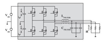
Fig. 8. Three phase DC/AC converter.
