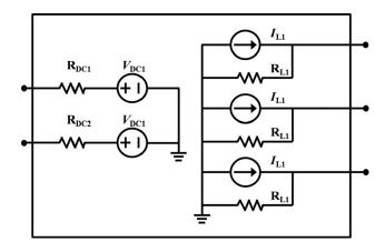
Fig. 5. DC/AC converter system solver structure.
